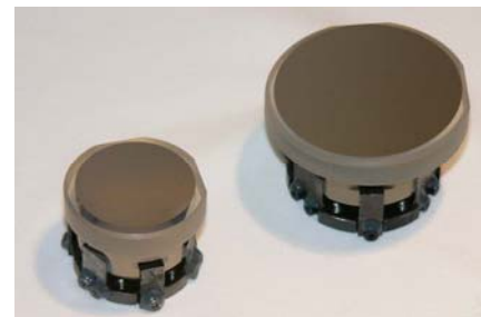
Fig. 7: One of the 2 sets of SWAP mirrors after coating
