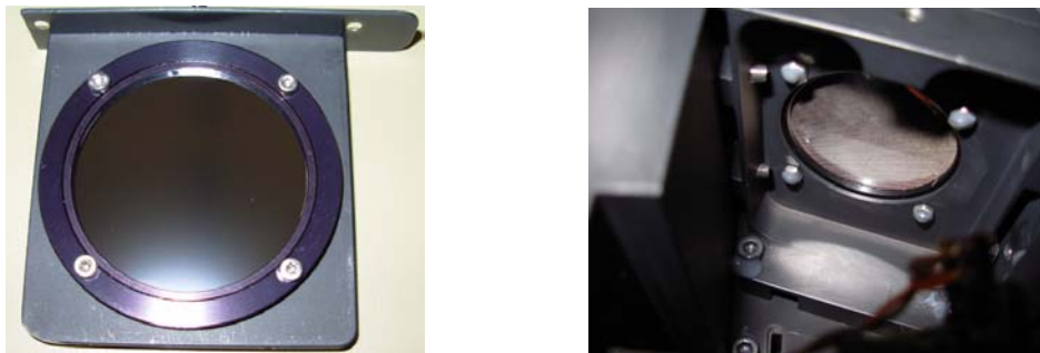
Fig. 8. SWAP front and rear aluminum foil filters
